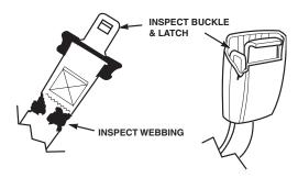
Figure 2-3. Seat Belt Inspection
